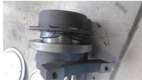
Issue detected: Broken membrane inside cooler valve
